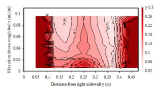
Figure 3. Contour curves of constant longitudinal velocity  $V_x$  (Top) and velocity vertical fluctuations  $v_z{}^{{}^{{}^{{}}}}$  (Bottom) with rough bed and rough sidewall -  $Q=0.0261\ m^3s^{-1},\ x=5\ m,\ y=0$  at right smooth sidewall, velocity scale in  $ms^{-1}$
