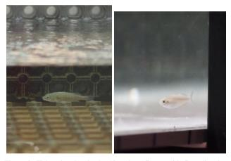
Figure 2. Fish swimming in the 12 m long flume, with flow direction from left to right. Left: juvenile Silver perch close to the rough sidewall; Right: Duboulay's Rainbowfish along the smooth sidewall
