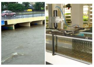
Figure 1. Physical modelling of culvert hydrodynamics. Left: prototype operation in Brisbane on 20 May 2009; Right: laboratory channel with rough bed and sidewall configuration
